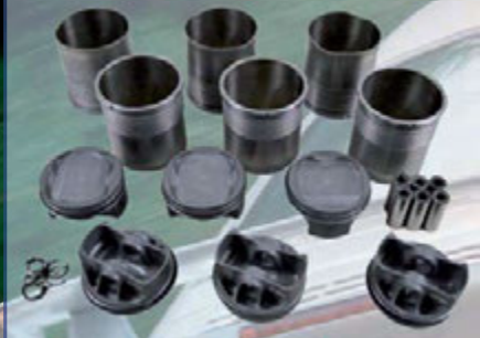
Mahle 4.1L Upgrade (9.1:1) Piston & Cylinder for 996/997 Turbo/GT2
